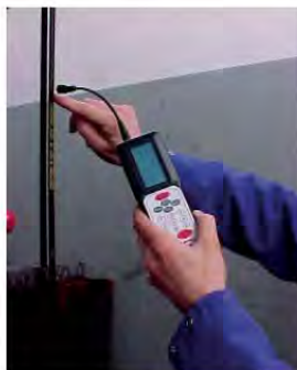
TENSION CONTROL BY VIBRATION METHOD
